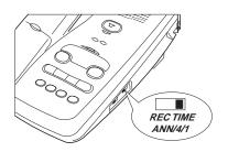
Four minute option: move the **REC TIME** switch to **4**.
